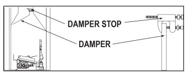
Use the 3" adjustable bolt to adjust the damper to the correct opening, based on the enclosed chart.
